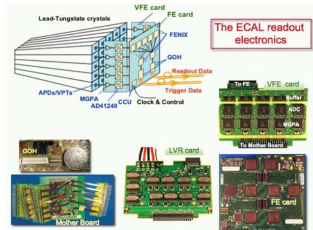
Fig. 6. Components of the ECAL readout electronics
