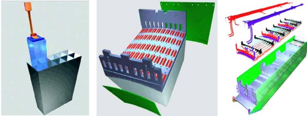
Fig. 5. Stages of an ECAL supermodule assembly. Left: Alveolar submodule during insertion of the first crystal; Centre: Complete module; Right: Expanded view of a supermodule with cooling circuits
