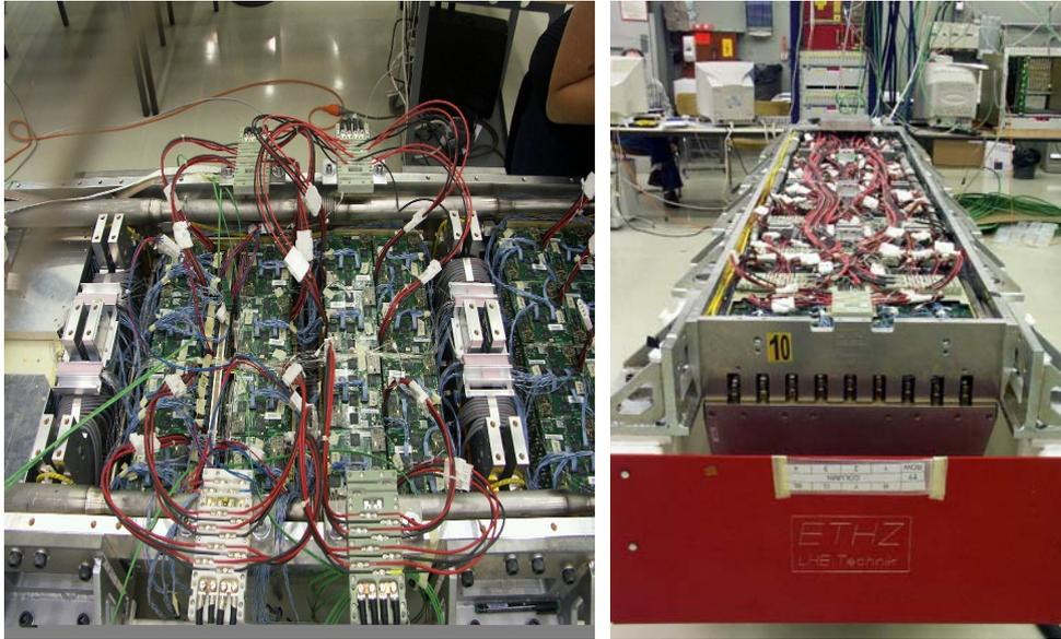
Fig. 7. Different steps during the integration of the readout electronics into supermodules
