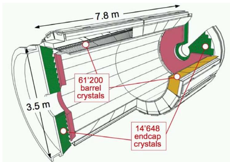
Fig. 4. Overall view of the CMS electromagnetic calorimeter
